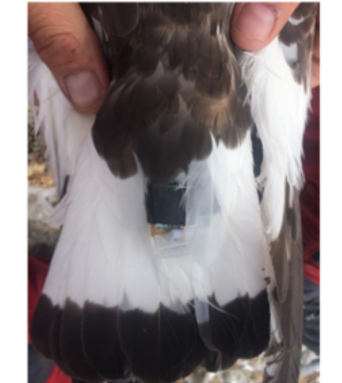
GPS logger attached to feathers with Tesa® tape
